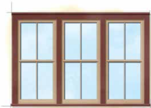
Double-hung window combination (exterior)
