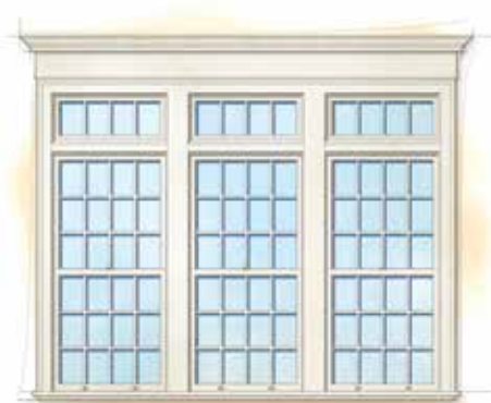
Double-hung and transom window combination (interior)
