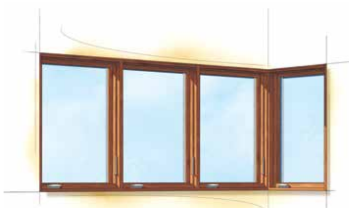
Casement and auxiliary window combination (interior)
