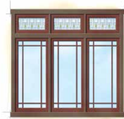
Casement and transom window combination (exterior)
