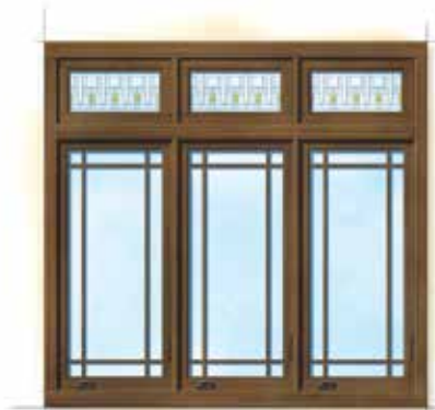
Casement and transom window combination (interior)
