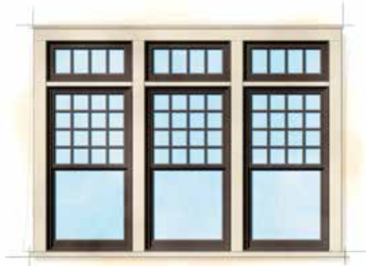
Double-hung and transom window combination (exterior)
